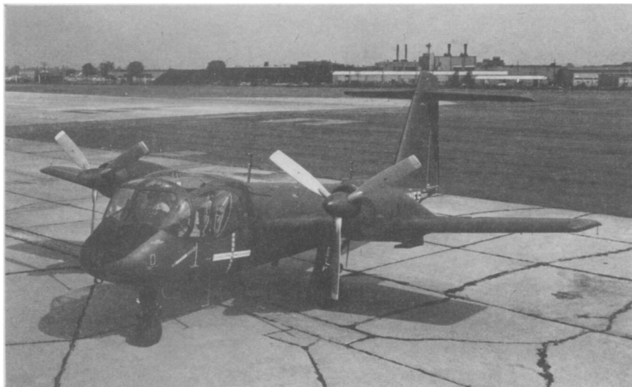
TURBO-PROP AIRCRAFT —A new observation plane, the U.S. Army's first turbo-prop powered fixed-wing plane, has been built by the Grumman Aircraft Engineering Corporation. The AO-1 Mohawk is designed to operate from small, unimproved fields, water, snow and mud; a bubble canopy provides maximum visibility.
