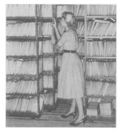
The wheeled base units, shown in the photograph, are adjustable in all directions to fit units ranging from 24 to 48 inches in width and 9 to 42 inches in depth. The load capacity of each unit is one and one-half tons.
