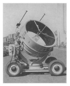
SOLAR FURNACE — Surplus military searchlights made possible the development of this sun-powered furnace now available on a mass production basis. The American Searchlight Corporation, New York, which produces the furnace, reports temperatures as high as 8000 degrees Fahrenheit have been reached with the furnace.
