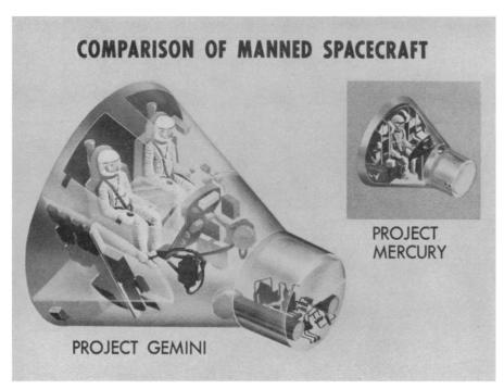
RENDEZVOUS CAPSULE—The two-man spacecraft Gemini, named for the twin stars Castor and Pollux, will be used to develop rendezvous techniques for joining parts of spacecraft sent aloft separately and for extended earth orbit missions lasting a week or more.
