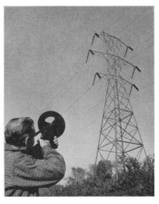
TROUBLE SHOOTER—An ultrasonic "gun" which detects corona, or leakage of high-voltage electricity causing static and loss of electric power, has been developed by Westinghouse Electric Corporation, Pittsburgh, Pa. W. E. Pakala tests a transmission line with the device.
