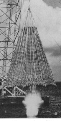
"OPERATION SNARE"—This device is used to test the advanced versions of the Navy's submarinelaunched Polaris missile. It enables technicians and engineers at Lockheed Missiles and Space Company, Sunnyvale, Calif., to study the missile's underwater performance. The bag of nylon webbing is suspended with its bottom open and waiting directly above the launch tube on the ocean floor. The bag catches the missile as it breaks the surface.
