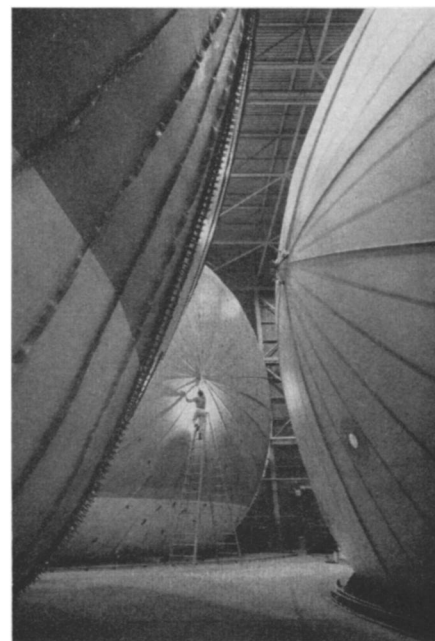
GIANT BALLOONS are actually transportable radar antennas developed by Westinghouse Corporation for the U.S. Air Force. Use of such antennas in space is under study.
