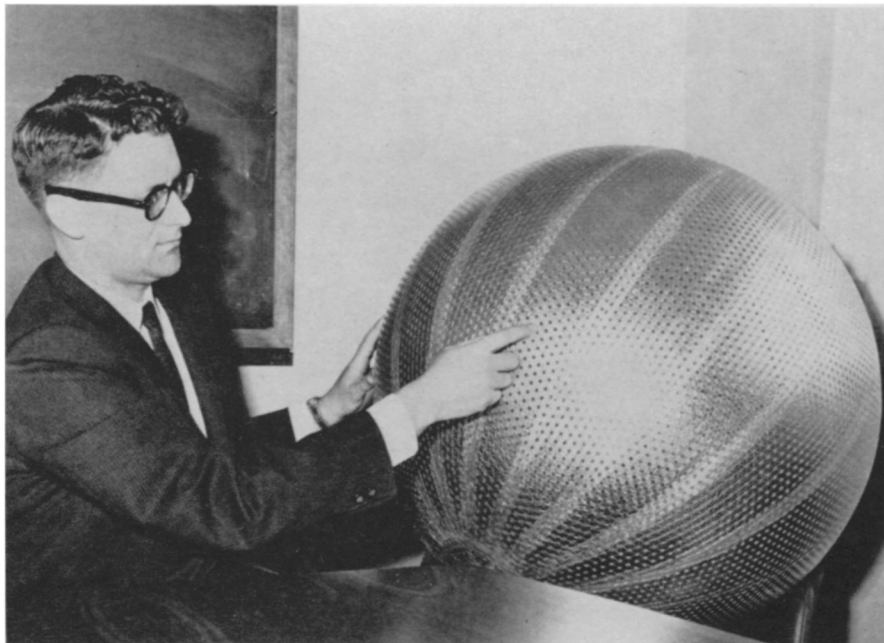
LIGHT-WEIGHT SATELLITE —Shown is an inflatable satellite model of aluminum and plastic foil weighing one-third less than materials now used. It was developed by Aluminum Company of America, Pittsburgh, Pa.
