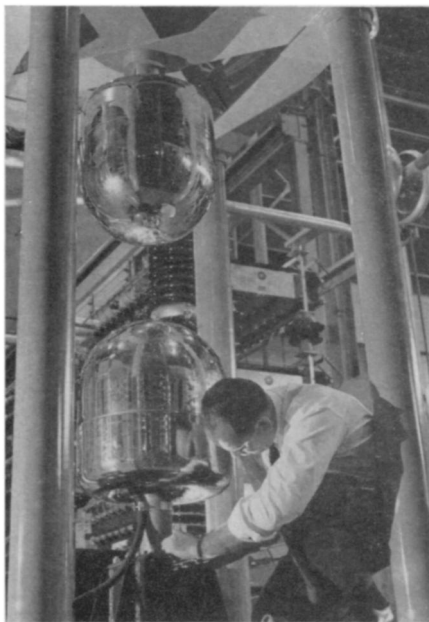
RADAR TUBE PROTECTOR —Performing the same job as a lightning rod on a home or a barn, a crowbar discharge switch developed by the Westinghouse Electric Corporation, Bloomington, Ind., protects expensive high powered radar tubes from damage. The switch will respond in eight millionths of a second.
