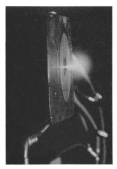
NEW WELDING METHOD-Electrons produce a bright glow as they emerge into the air from the new apparatus for electron beam welding in inert gas. The electron beam and workpiece are enveloped in a continuous flow of inert gas during the welding process.
