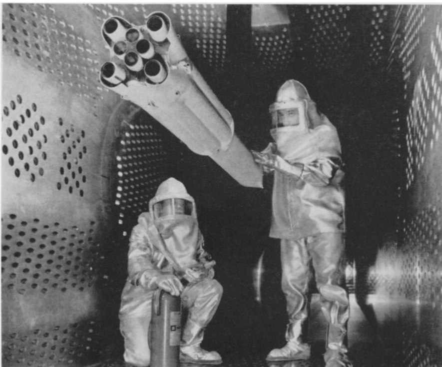
PLANET PROBE MODEL —Technicians of the National Aeronautics and Space Administration check out a model of the Saturn rocket before a supersonic wind tunnel run. The Saturn booster may send probes to Mars and Venus.
