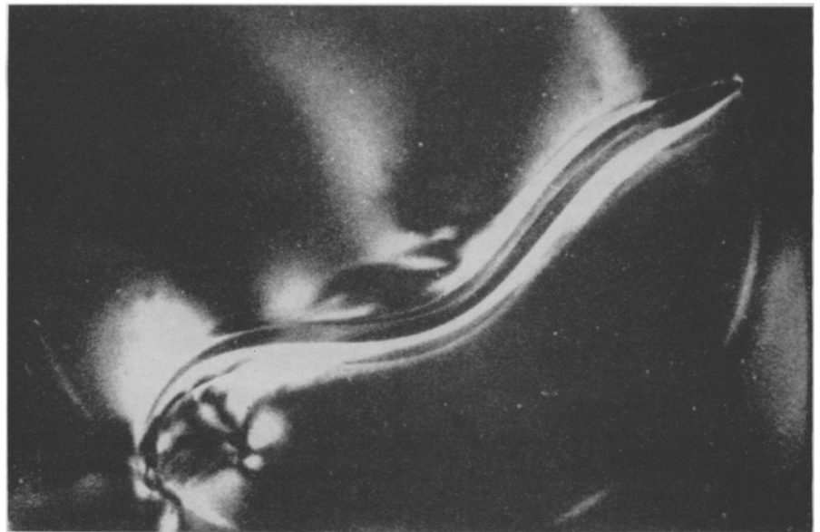
BIONICS RESEARCH —An eel is seen swimming through a bentonite-liquid mixture during studies of hydrodynamic design.
