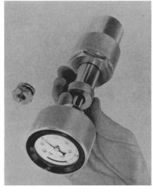
PORTABLE PULL TESTER is a hydraulic instrument about the size of a flashlight for use in checking the holding power of threaded fasteners of one-fourth or threeeighths-inch in diameter. Precision-built, the instrument can subject a completed fastening to stresses up to 5,000 pounds. The device weighs only two and one-half pounds as compared to ordinary testers weighing 50 to several hundred pounds.
