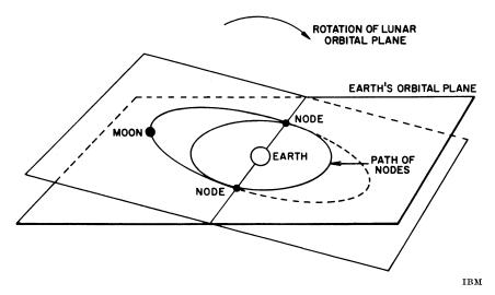
MOON'S ORBIT RECALCULATED—The diagram shows the path of the moon's orbit around the earth and points where the moon intersects the plane of the earth's orbit, the nodes. Astronomers have found that the motion of the moon's nodes is a sensitive indicator of the forces acting on the moon. Lunar theories can be tested by comparing the theoretically calculated motion of the nodes with the observed motion.
