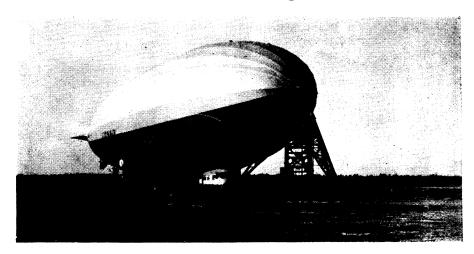
changes, the craft can be brought very close to the ground without danger and made easily accessible for repairs.
