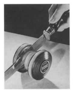
motion of the knife rotates the spool, putting a keen edge on the blade.
