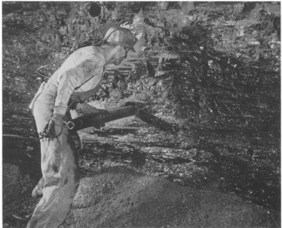
AIR BLASTING —A new safety feature in mines is this modern air-blast shell which a miner is inserting into a wall of coal. The air shoots into the shell through the copper tube which leads back a safe distance from the site of the blast and will send about 35 tons of coal crashing out of the vein.
