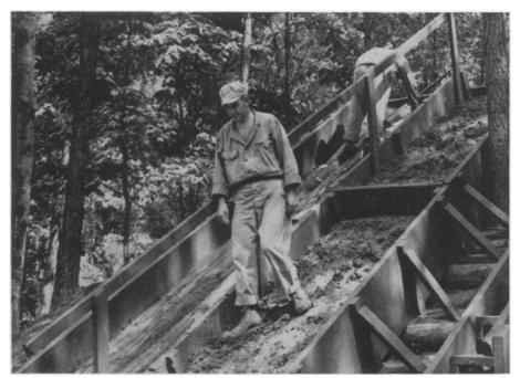
TESTING GI SHOES—Longer-wearing footwear for civilians and Army is expected from the experiments made at the shoe track at Camp Lee, Va. Here a soldier is shown in the process of testing new shoes on mud and log traction slides. As a result of this program a type I leather-soled shoe was found early in the war to last 150 miles while a recent type III shoe, using synthetic rubber material in the sole, has a life expectancy of 2,500 miles.
