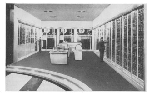
VAST MEMORY CAPACITY—This new electronic calculator can remember and recall automatically 400,000 digits. Its speed, memory capacity and flexible and convenient programming facilities will make it especially advantageous in the realm of science.
