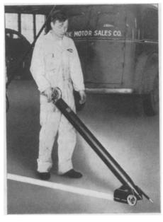
of the device, shown in the picture, holds six quarts of paint which is released by a finger-grip trigger.
