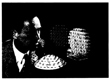
NEW TYPE METAL LENS—It will be used for focussing radio waves in radio relay systems in the way an optical lens focusses light. It is theoretically capable of handling from 50 to 100 television channels or tens of thousands of simultaneous telephone messages, in the proposed radio relay link the Bell System is planning between New York and Chicago. Shown with three different small-scale models of the lens is Dr. Winston E. Kock who developed them.
