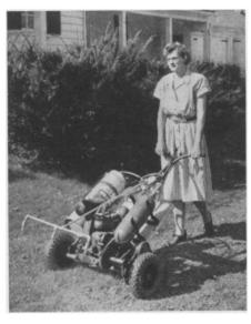
killing chemicals or insecticides to lawns, is attached to the lawnmower as shown in the picture and uses a tank of compressed carbon dioxide gas instead of the pump usually used in spray units. The combination sprays as it mows.
