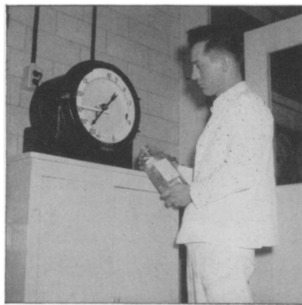
Recorder, measuring electrolytic conductivity
