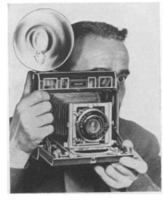
AERIAL FRAME viewer on a new type camera permits the photographer to use both eyes, one looking through the focusing window, the other with unobstructed view as shown in the picture. Focusing through the rangefinder is first made with one eye; then both are used to keep the picture framed and observe the subject's actions at the same time.
