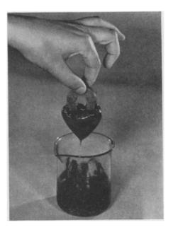
MAGNETIC FLUID—It consists of a mixture of fine iron powder and oil which forms the heart of the NBS magnetic fluid clutch. When acted upon by a small permanent magnet, that portion of the mixture in the magnetic field "solidifies", as the iron particles become mutually attracted, and adheres to the magnet.
