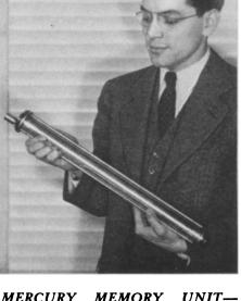
MERCURY MEMORY UNIT— The mercury tube shown here being held by Isaac L. Auerbach, one of the men who perfected it, is the core of the new memory system in which a thousand numbers can be stored. Just revealed, it is said to be ten times as fast as former methods.
