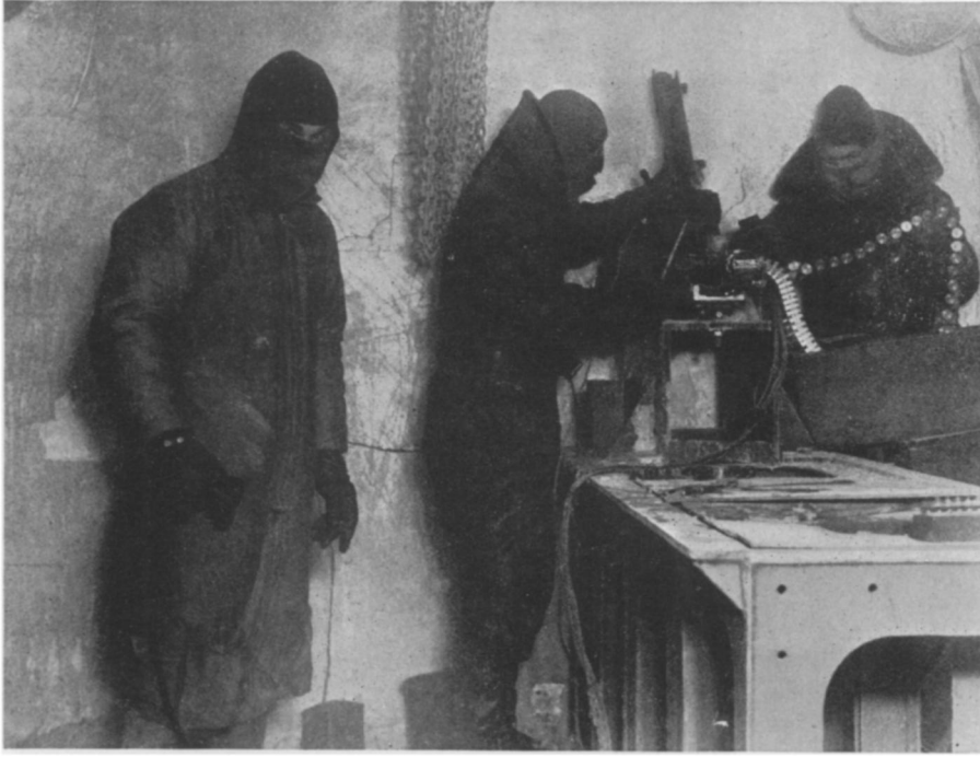
TESTING GUNS IN EXTREME COLD —Braving 70-below-zero cold to test guns and ammunition, these Navy ordnancemen are loading a 50-caliber machine gun. Almost all gear is electrically operated by remote control. The suits worn by the men contain electric heating units and the guns are fired through quick opening ports.
