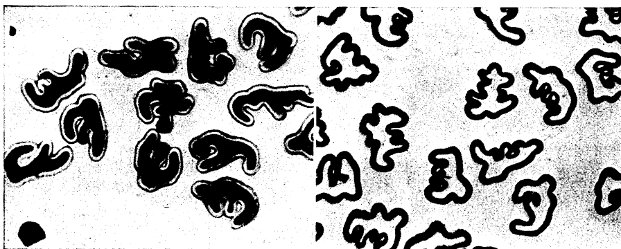
RAYON DYE PROCESS —These are cross-sections of rayon fibers showing, on the left, that the core absorbs the dye before the skin, and, on the right, that dye washes out of the core more quickly than from the skin.
