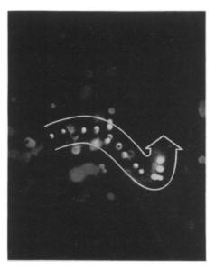
ELUSIVE ELECTRON—The first definite tracks of electrons, particles that make up atoms, are shown in this picture, developed after an electron sped through the emulsion, striking silver grains in its path. This shows an enlargement of a 13-grain track. X-rays, filtered through lead, were used to start the electrons flying into this new type of Eastman plate.
