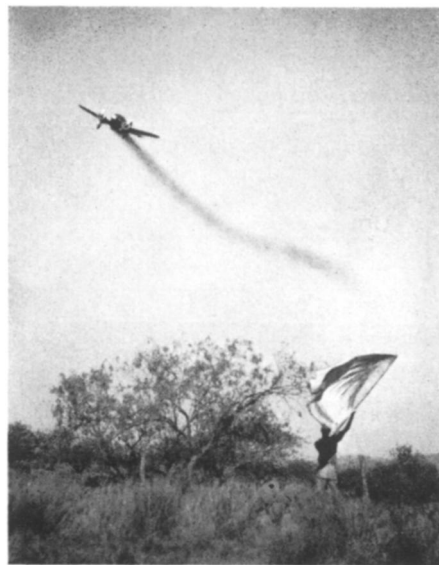
AERIAL SEEDING —At a signal from the flagman, the pilot pulls the trigger which releases seeds. The seeds are pellets being dropped over grazing land in Arizona.
