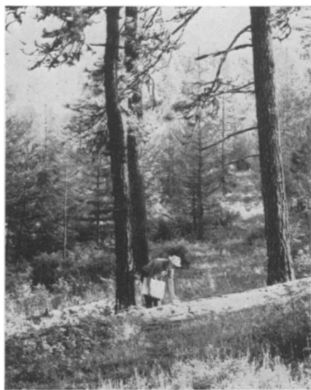
EFFECTIVE TEST —Glass plates set at right angles to the path of the spraying plane pick up samples of droplets and thus give an idea of effectiveness of the attack.
