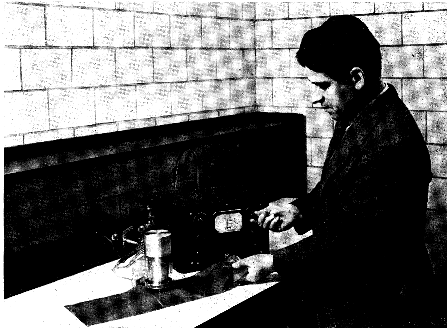
UNIQUE MEASURING DEVICE —A gauge for measuring the thickness of thin rubber and other thin films on continuous production equipment, has at its heart a radioactive isotope, byproduct of the nation's atomic energy plants. Shown in the picture is W. E. Morris, who developed it in the research laboratory of the Goodyear Tire and Rubber Company. It is capable of measuring material as thin as one-thousandth of an inch.
