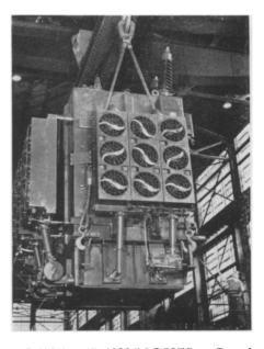
GIANT TRANSFORMER — Rated at 110,000 kilovolt-amperes, this powerful machine can handle enough power to fill all the electrical needs of an average city of 200,000 persons.
