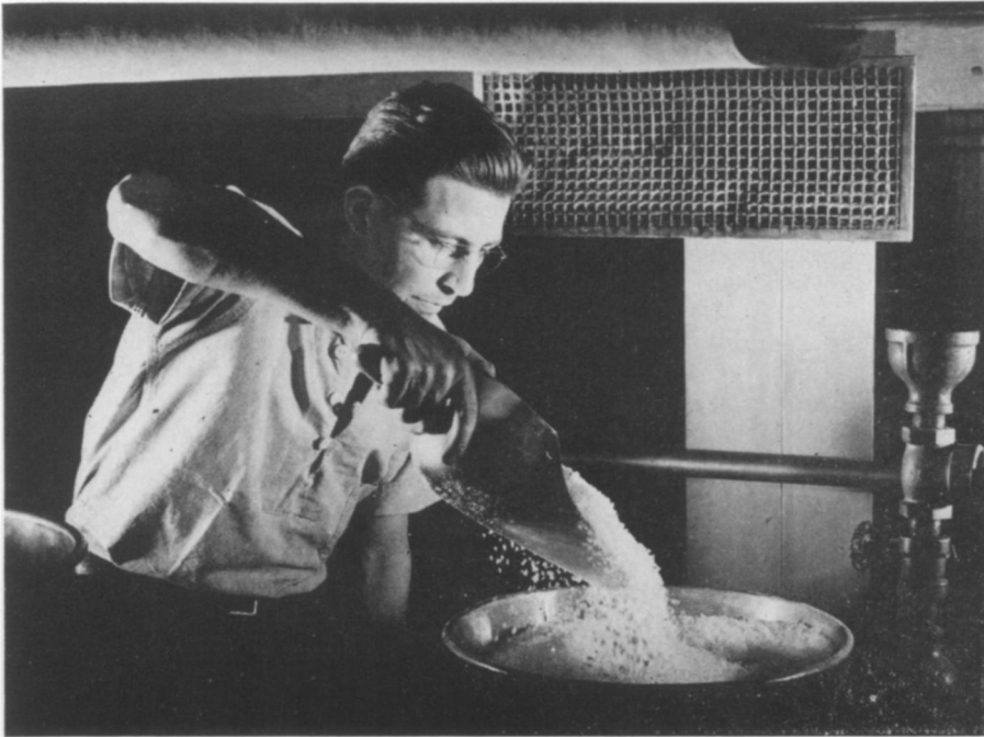
NYLON FLAKES —This shows them being fed into the hopper of a spinning machine where the flakes are melted and extruded into filaments.
