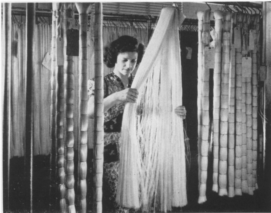
HANKS OF NYLON —These will be used for bristles in tooth, hair and industrial brushes. They are inspected as they are tied up in preparation to being cut into bristle lengths.
