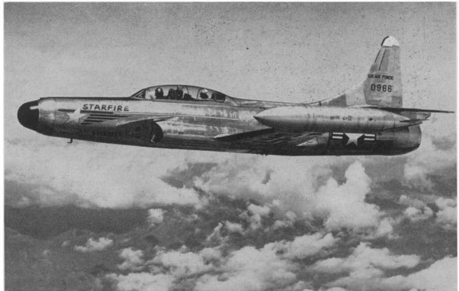
THE SUREFIRE STARFIRE —The all-rocket-armed F-94C pictured above is now being delivered to the U. S. Air Force by Lockheed Aircraft Corporation. Loaded with radar and electronic equipment, the jet interceptor can shoot down invaders with its 24 rockets without its crew ever seeing the enemy.
