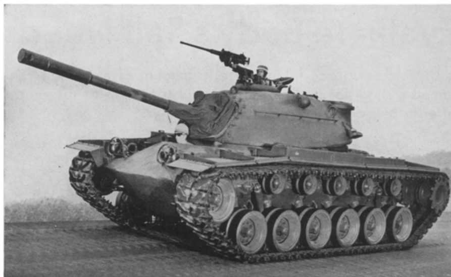
ARMY'S NEWEST TANK —The Patton 48, the most modern medium tank, has a one-piece, cast-armor hull and improved firepower to make it a formidable fighting machine.
