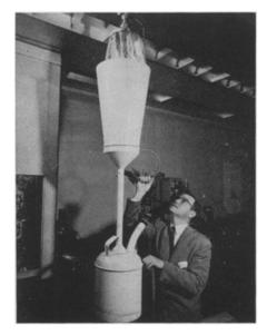
testing showers installed to quench clothing fires that might occur in the laboratory. A vertical assembly funnels water from the sprinkler into a can, as shown in the photograph, and a connecting hose carries the water to a nearby sink, thus protecting the clothing of the testing engineers.
