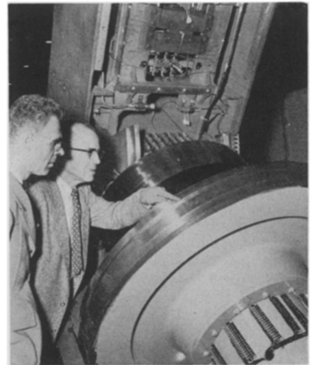
CORONAGRAPH MOUNT —The polar axis shaft for one of two new coronagraph mounts is here being inspected by Dr. John S. Evans, superintendent of Harvard's Sacramento Peak Station. Demonstrating the new mount is S. Dale Phillips, engineer in charge of production of the mounts.
