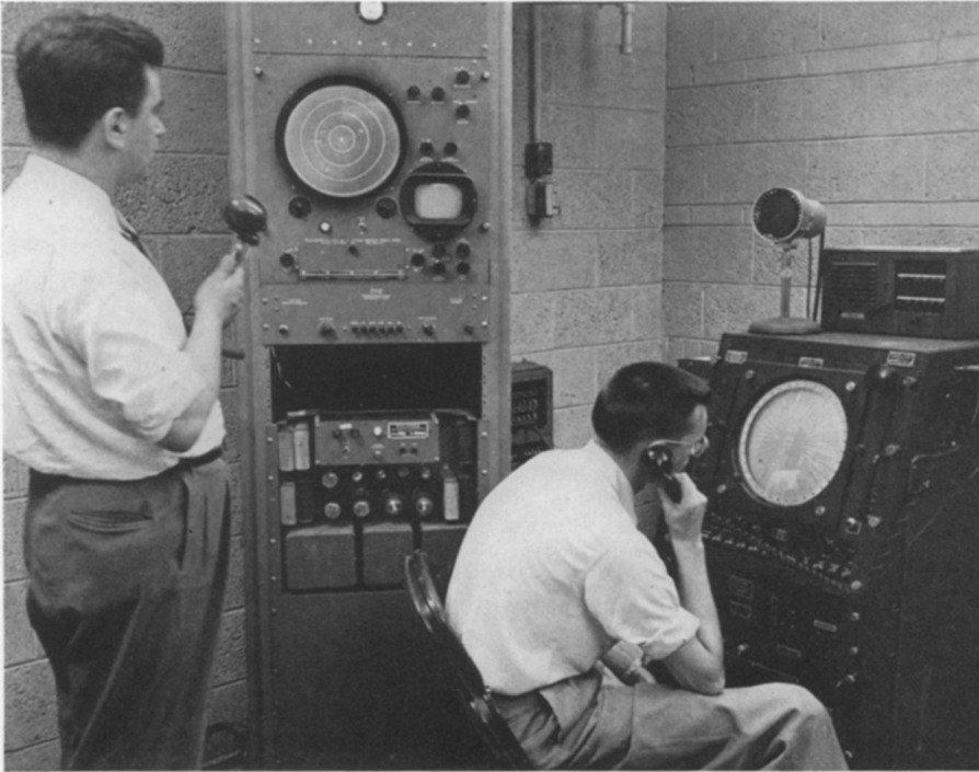
RADAR-TELEVISION COMBINATION — Spotting planes approaching airports is easier using the bright-tube screen that shows the pips more clearly under normal room light.
