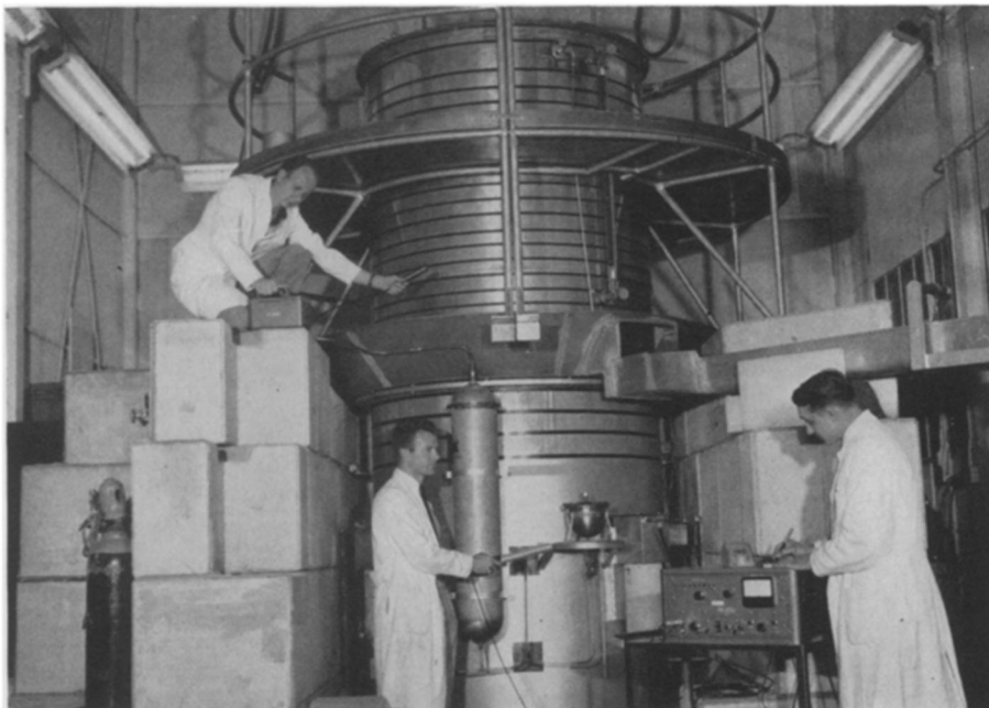
WATER BOILER REACTOR —This “baby” reactor, designed and built by North American Aviation to run on less than one watt of power, is being used to learn more about reactors. The shielding concrete blocks have been removed to show the tank-line housing where the graphite reflector and core are located.
