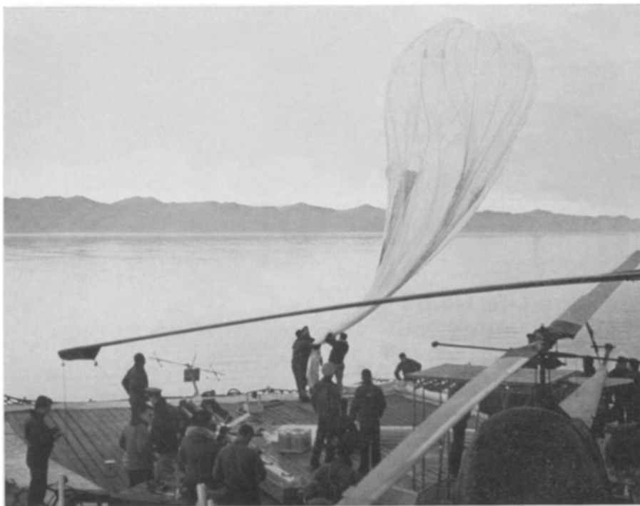
DAWN LAUNCHING —This cosmic ray balloon is being released from the deck of the Eastwind near Cape Parry off the Greenland coast. The purpose is to measure cosmic radiation in the vicinity of the northern geomagnetic pole.
