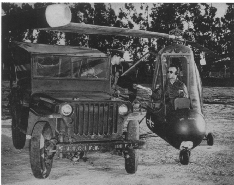
JET-POWERED, ONE-MAN HELICOPTER —In contrast to the giant shown on the cover, the Army's XH-26 is a jet-powered, one-man, collapsible helicopter. The baby craft weighs less than 300 pounds.
