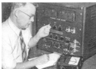
Dynamic Fluxmeter, developed by Bell Telephone Laboratories, indicates flux build-up in intervals of 25 millionths of a second. Precise information like this was essential to higher speed operation.
