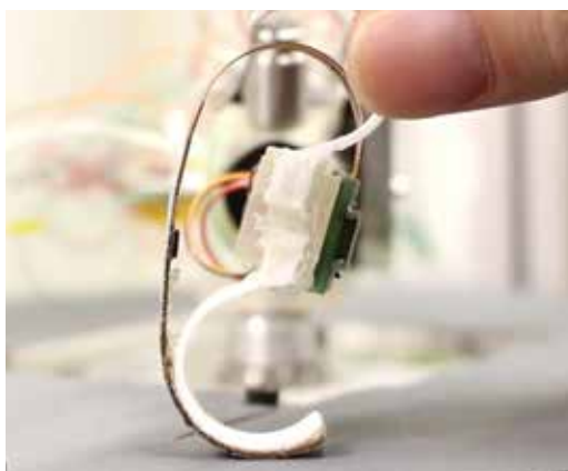
A small running robot named SAIL-R (top) has tactile sensors attached to six C-shaped legs (left). When the legs whirl around and smack the ground, the sensors detect the impact forces, which could help the machine choose an appropriate walking gait.
