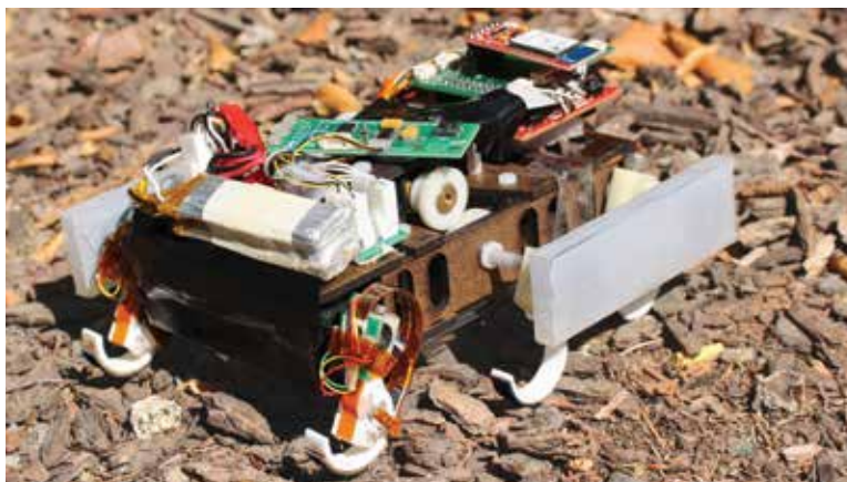
A small running robot named SAIL-R (top) has tactile sensors attached to six C-shaped legs (left). When the legs whirl around and smack the ground, the sensors detect the impact forces, which could help the machine choose an appropriate walking gait.
