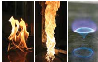
A swirling flame is produced in the lab by igniting fuel floating on top of water (left). The flame transitions into a fire tornado (center) then settles into an efficiently burning blue whirl (right).
