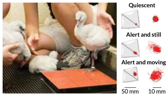
A young flamingo sets one foot on an instrument that tracks posture. The smallest shifts (red squiggles, right) in the foot's center of pressure, where weight is focused, occur when the bird is quiescent. For active birds, shifts are bigger.
