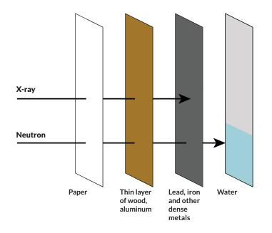
**See through** Scientists rely on X-ray and neutron scanning to penetrate materials that hide objects of interest. Differences in how X-rays and neutrons interact with atoms explain why neutrons, unlike X-rays, can pass through lead but get blocked by water.
