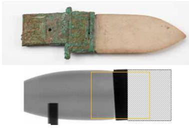
In a test of how neutron imaging might work on a 3,000-year-old jade dagger-axe from China (top), researchers at the Freer Gallery of Art made a replica using jade, stacks of brass plates and silk thread. In an X-ray of the replica (middle, shown facing the opposite direction as the real artifact), the haft is completely obscured by brass. Imaging a portion of the replica (area outlined in yellow) with neutrons revealed hidden details (bottom).
