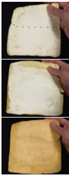
This vegan leather contains dormant fungal spores. When the leather gets a hole (top), spores can be revived to mend it (middle). But repairs remain visible (bottom).
