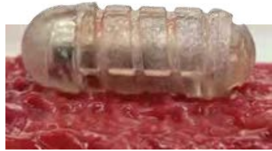
RoboCap, shown resting on a pig intestine, can sweep away mucus in the gut and leave behind drugs to be absorbed by the body.
