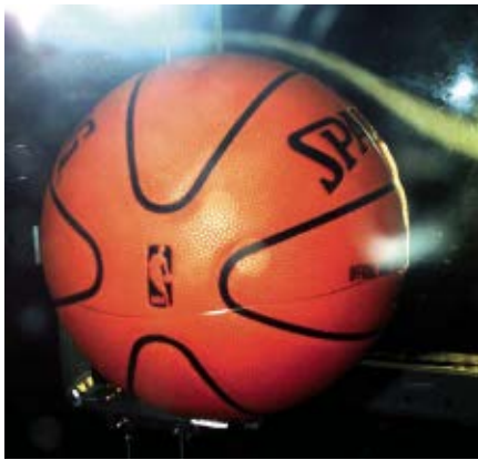
AIR BALL A plastic basketball that's now the official ball of the National Basketball Association undergoes wind tunnel testing.
